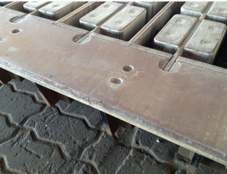
Figure 1: Segmented cover plates for simplified exchange of wearing parts.
