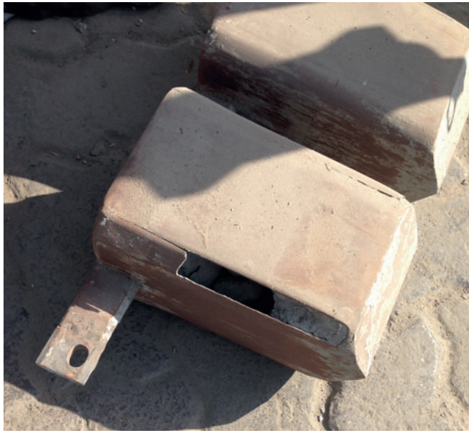
Figure 5: Nitrated core, totally worn out
