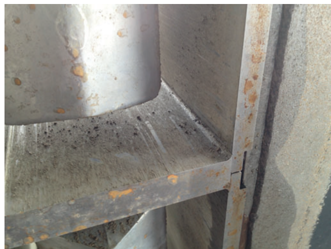
Figure 4: Minimal corner wear in a carbo-hardened Kobra hollow block mould.
