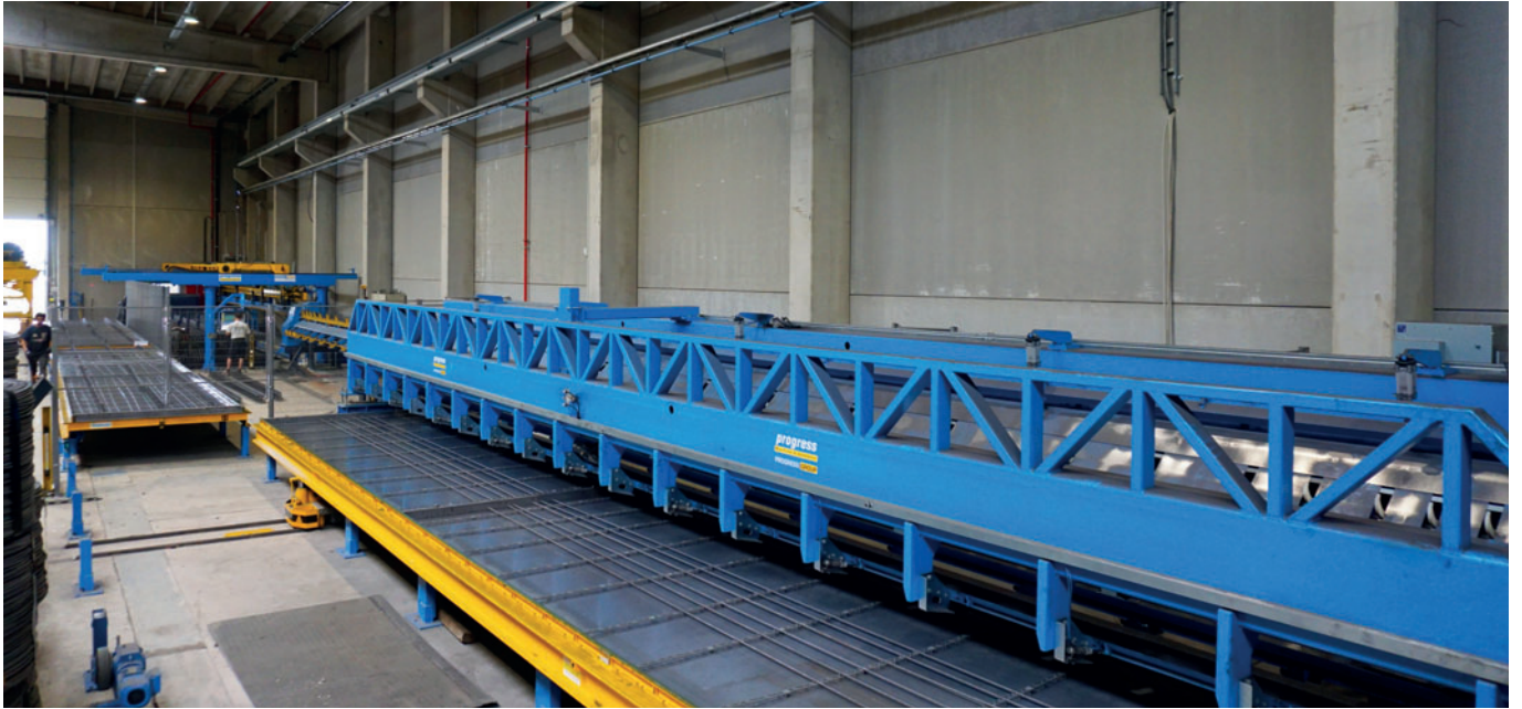
The pallet itself moves transversely below the run-off of the recently installed MSR straightening and cutting machine, in order to incorporate the longitudinal bars in their correct position.
