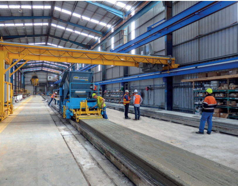
The Universal Slipformer allows Westkon Precast to manufacture hollow core slabs 20 to 50 cm in height.
