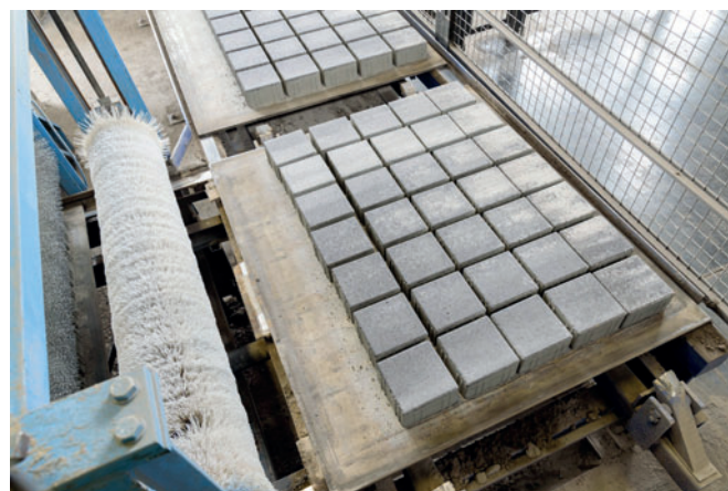
Following the period in the drying chamber, the blocks are brushed off once again and are then ready to be palletised.
