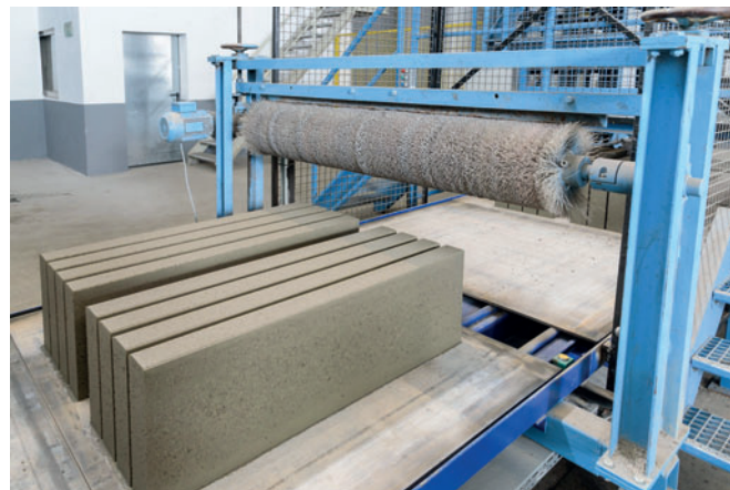
The concrete blocks can be brushed off if necessary after leaving the block making machine.
