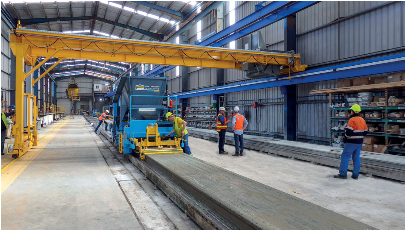
The Universal Slipformer allows Westkon Precast to manufacture hollow core slabs 20 to 50 cm in height.
