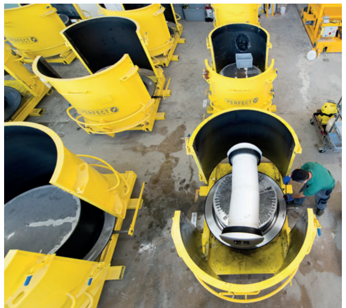
The negative EPS channels are inserted into easy-to-operate moulds and produced overnight in the mould
