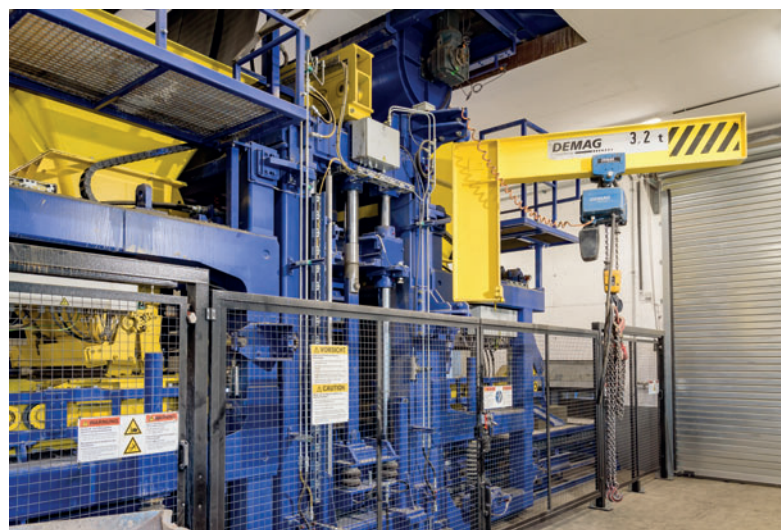
The main components of the XL 9.1: The compaction unit is located between the two filling units for core and facing concrete.
