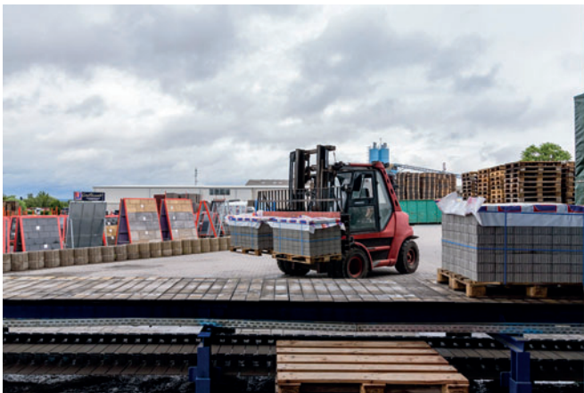
The pavers are stored on wooden pallets and provided with a protective film.
