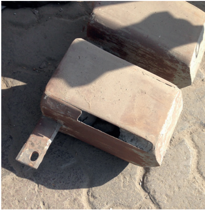
Figure 5: Nitrated core, totally worn out
