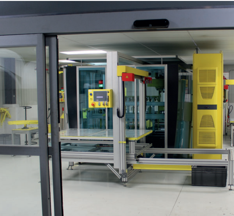
The heart of Perfect concrete manhole base production: The cutting center with 2D and 3D saws
