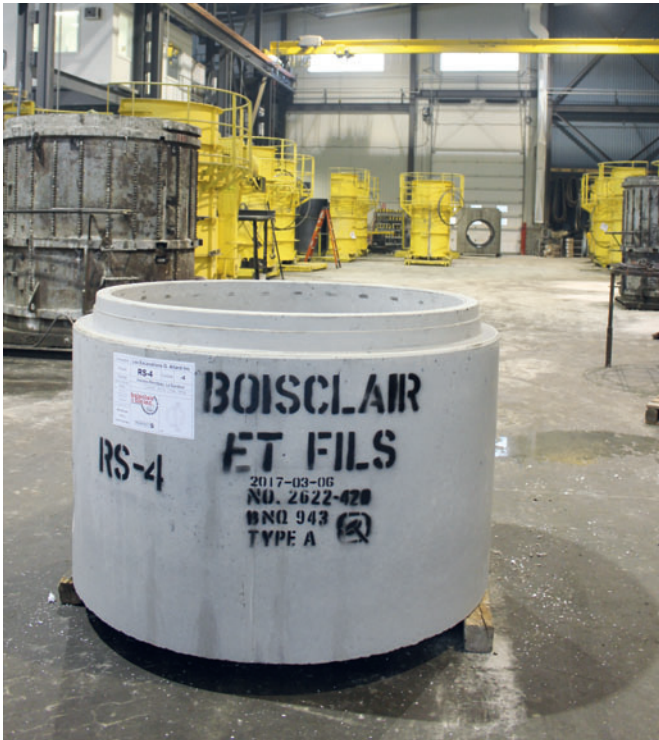
Finished Perfect concrete manhole bases before transfer to the external storage area
