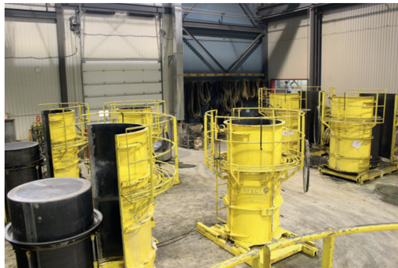
Mold station for the production of Perfect concrete manhole bases
