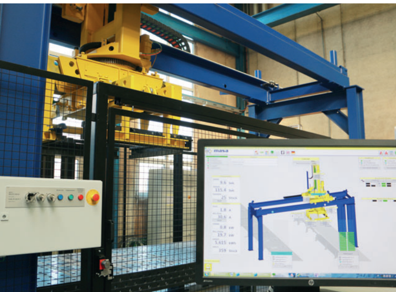
Fig. 9: A cycle time of 9.6 seconds was realised in the test setup
