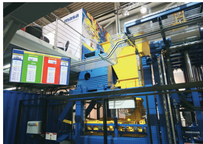
Fig. 3: Energy efficiency monitoring of the Masa XL concrete block making machine at the bauma 2016
