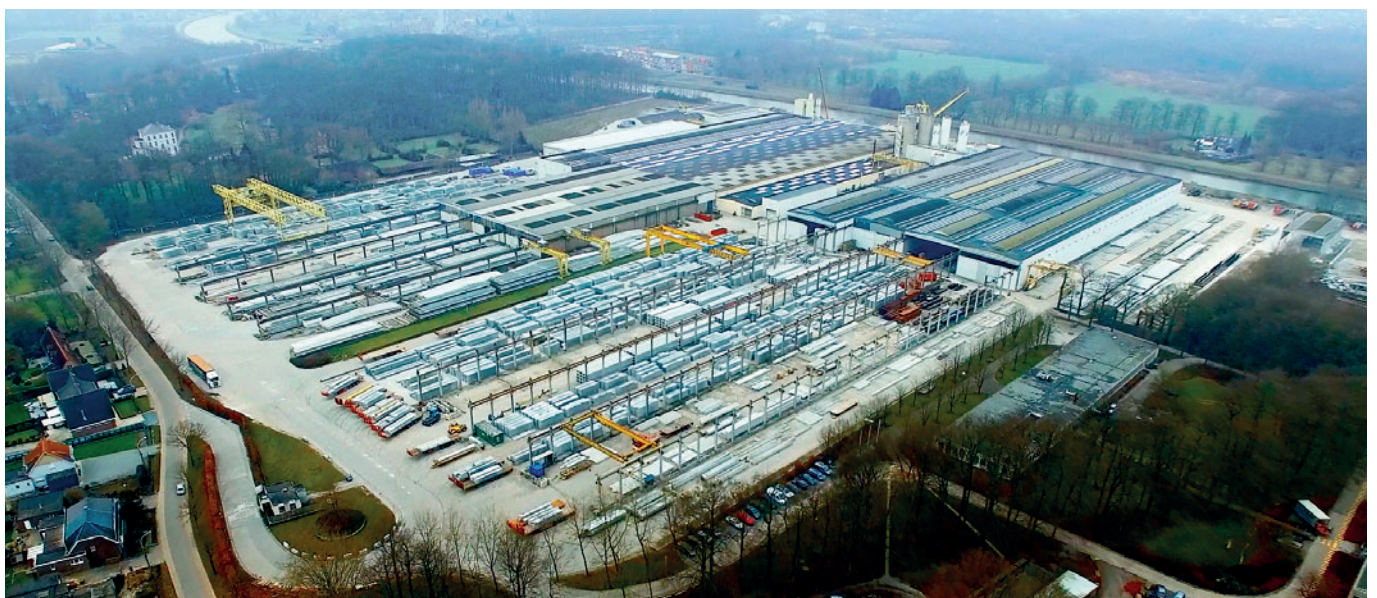
Factory grounds totalling 49,000 m 2 structural precast concrete elements, wall elements and hollow core slabs are produced. The total works site of the company, founded in 1963, covers a surface of 240,000 m 2 .
