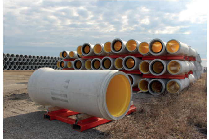
Con Cast Pipe has built special frames where the pipes are placed for storage and subsequent transportation to the construction site
