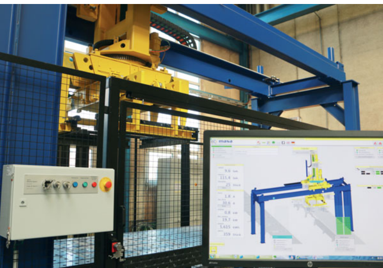
Fig. 9: A cycle time of 9.6 seconds was realised in the test setup
