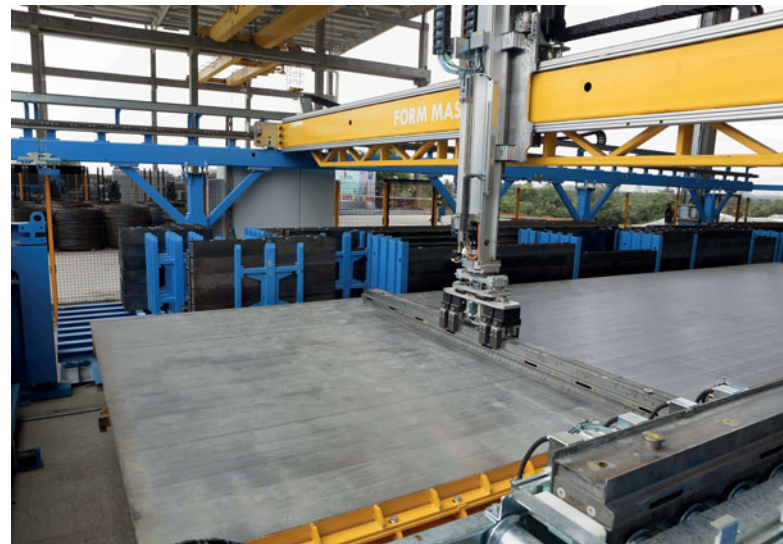
Shuttering and deshuttering have also been automated. This not only improves the quality of the end products and the rate of production, it also increases safety at work.
