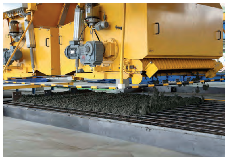
An automatic concrete spreader places the fresh concrete precisely and at a steady rate on the pallet.
