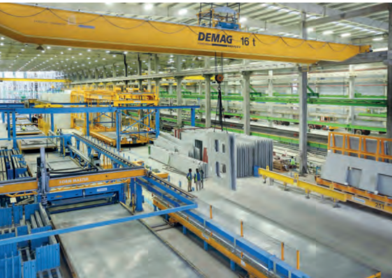
Fast and of high quality: KEF Infra manufactures various wall elements using the recently installed highly-automated carrousel system.
