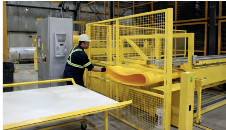
The fully welded liner is ejected from the welding machine and removed by an employee
