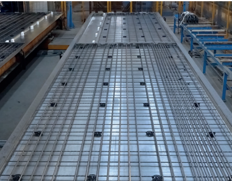
The spacers are placed accurately and a steady rate of concrete coverage is thus guaranteed. The savings potential is considerable.
