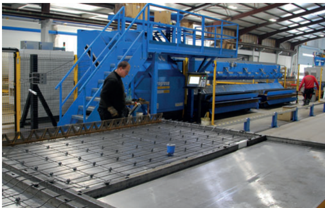
A straightening, cutting and bending machine of the type MSR16 BK was integrated into the carousel. Like the lattice girders, the bars produced are inserted manually.
