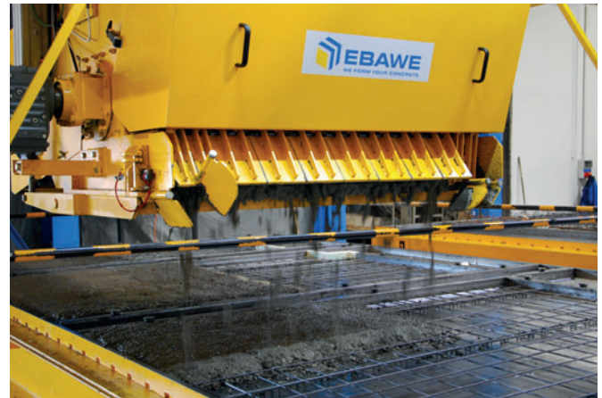
The fully automatic concrete distributor ensures that the fresh concrete is discharged accurately and evenly.
