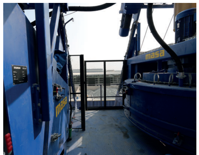
The new plant is equipped with two Masa concrete mixers: Masa mixer PH 2000/3000 (right) and Masa mixer S 350/500 (left)
