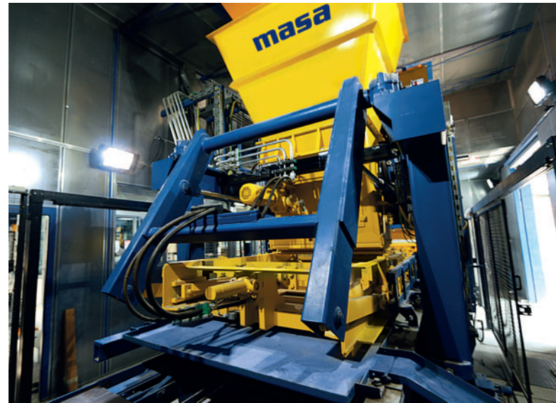
The heart of the new plant: Masa concrete block making machine XL 9.1
