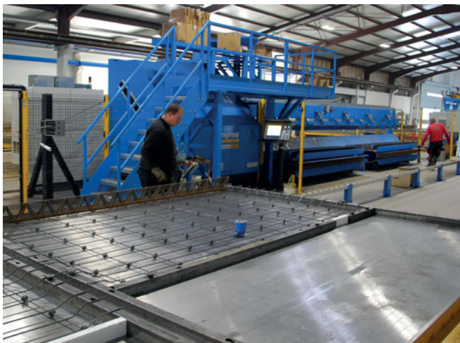
A straightening, cutting and bending machine of the type MSR16 BK was integrated into the carousel. Like the lattice girders, the bars produced are inserted manually.
