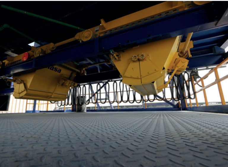
The ready mixed concrete will be transported to the block making machine by a double bucket conveyor
