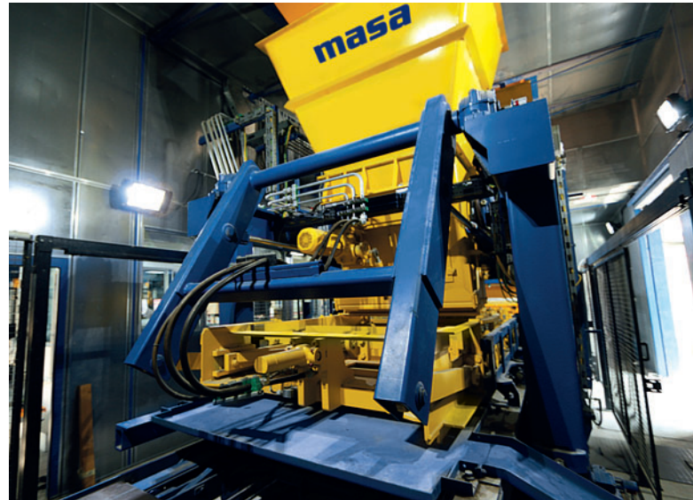
The heart of the new plant: Masa concrete block making machine XL 9.1
