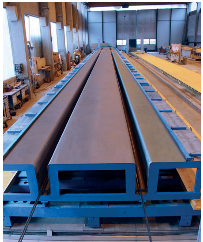
Tecnocom developed a flexible mould system with two different types of moulds for the Schachen plant: with the first, a 46 metre-long mould for the manufacture of TT slabs, the corresponding precast concrete elements are currently being produced.
