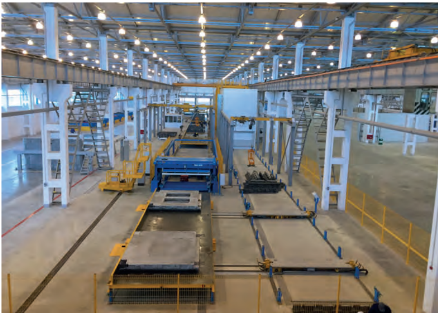
Solid and sandwich walls are manufactured on two carrousel plants (the picture shows the one in Ashgabat).
