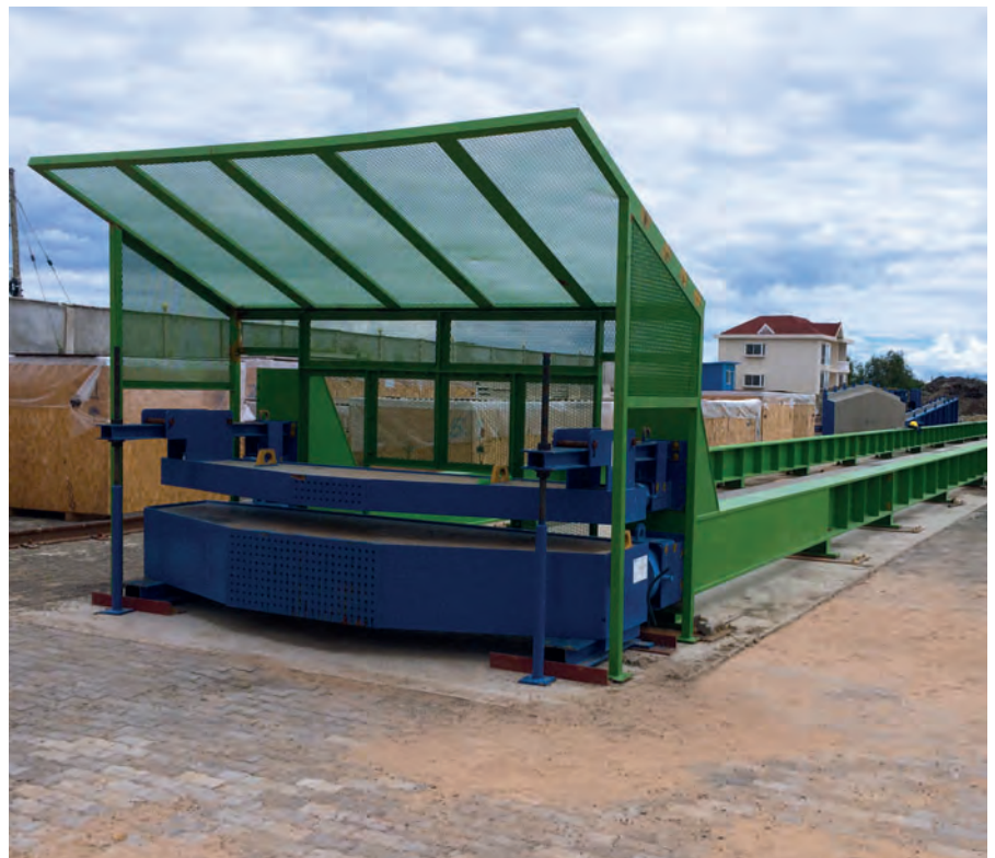
A mould with a self-stressing system for preloaded stresses can be fitted with various lateral shutters and insets. This allows flexible production of various types of beams.
