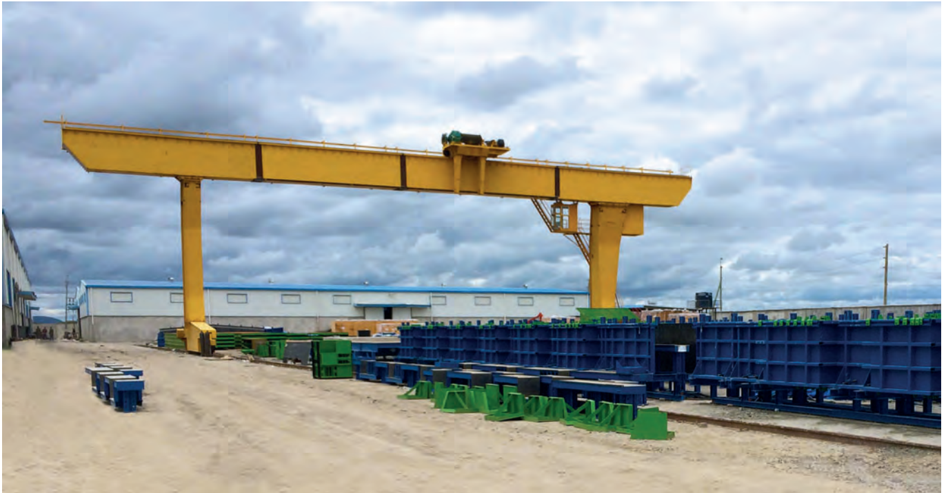
A total of six moulds, each 18 m long, are used for the manufacture of columns for commercial construction.
