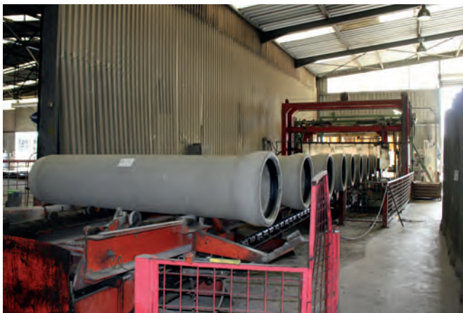
Inspection line for the finished pipes
