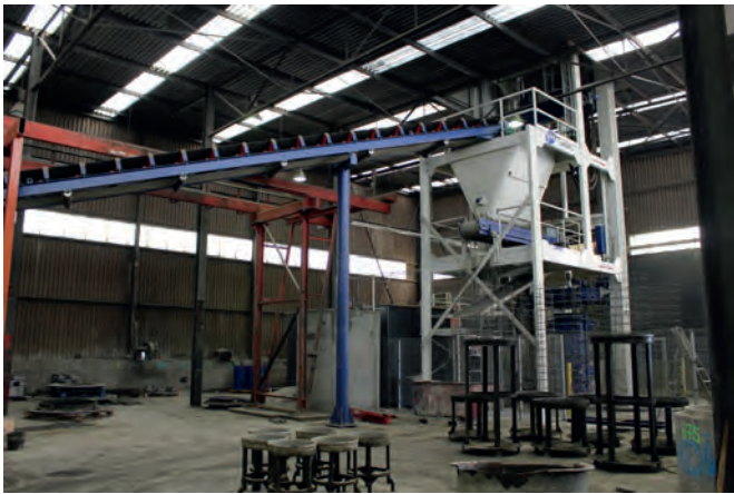
Concrete feeding to the RP 1630
