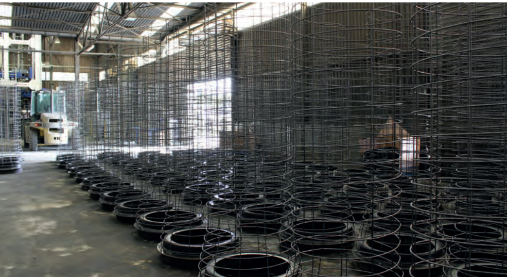
Base pallets with reinforcement stand at the ready
