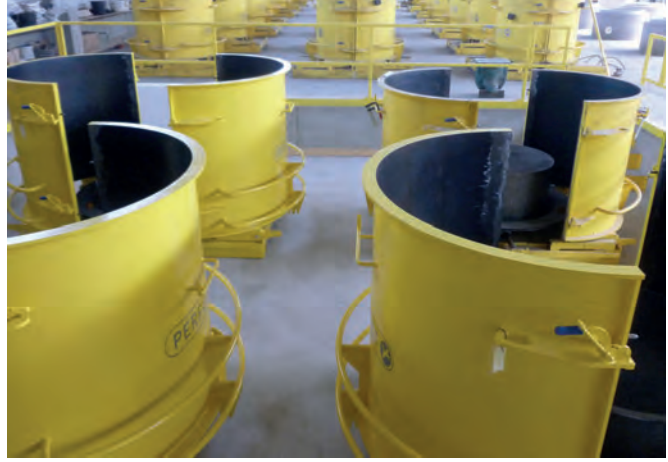
User-friendly steel moulds for manufacturing wet-cast concrete components with individually customised channel configurations.
