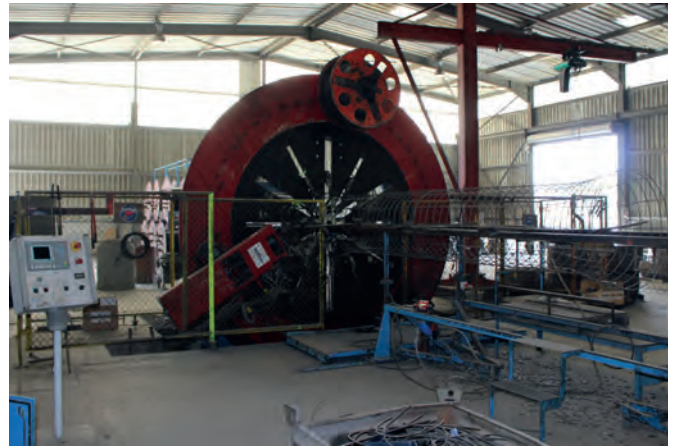
Apilion wire cage welding machine type ASMS
