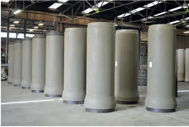
Freshly manufactured DN 700 pipes produced with the RP 1630
