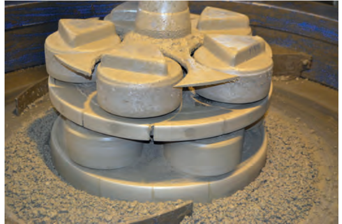
Counter-rotating compaction tool/packerhead
