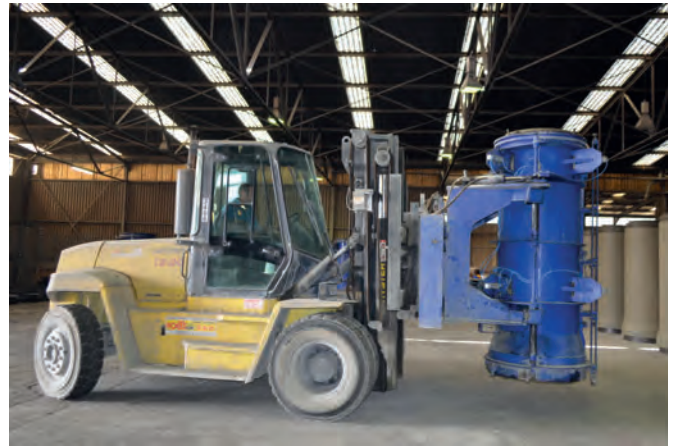
Fork-lift truck with a 3-part mould jacket
