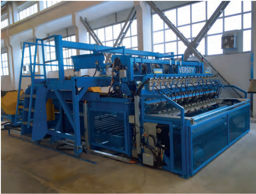
A mesh welding machine of the type Versity was installed in each of the modernised plants for the production of standard meshes. Stirrups and bars are produced on 9 additional machines.
