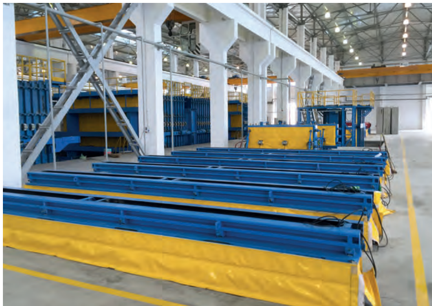
Beams (foreground), stairs (centre of picture) and ventilation shafts (background) can be produced using additional moulds, of which there are 15 in total. An integrated heating system accelerates the curing of the concrete.
