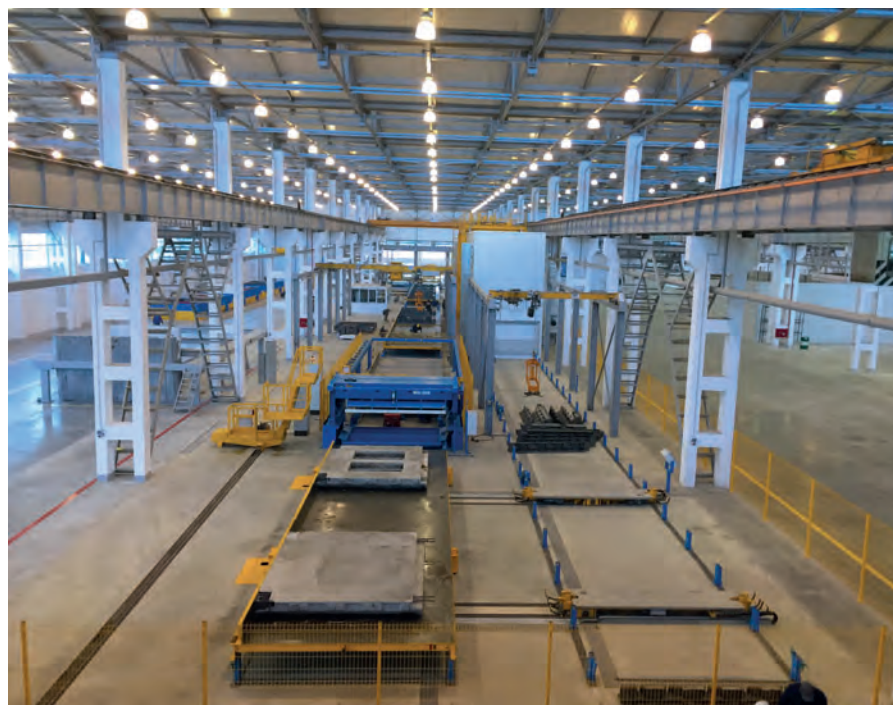
Solid and sandwich walls are manufactured on two carrousel plants (the picture shows the one in Ashgabat).
