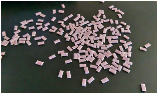
The granulate is available in a rectangular form and consists of LDPE (polyethylene), which is recycled from packaging materials
