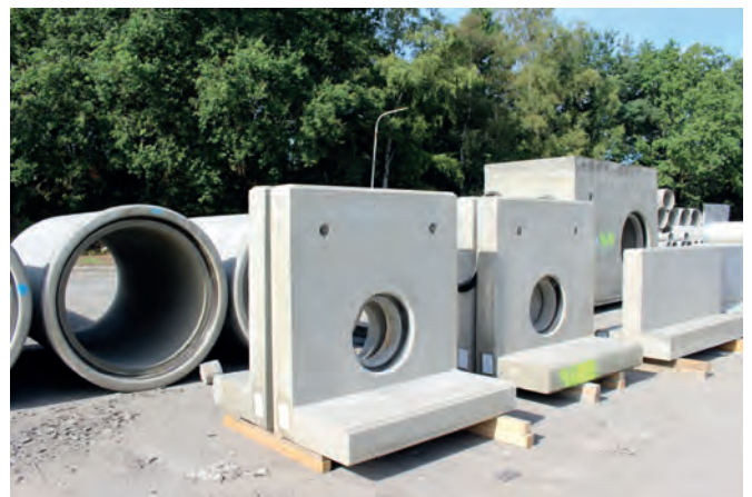
Retaining wall elements
