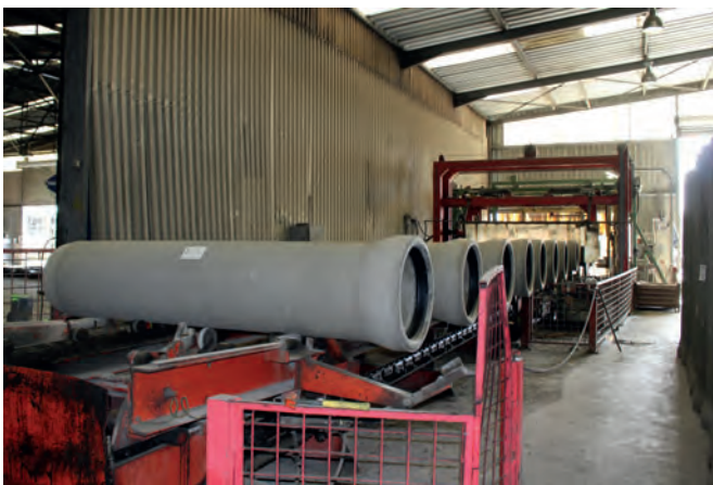
Inspection line for the finished pipes
