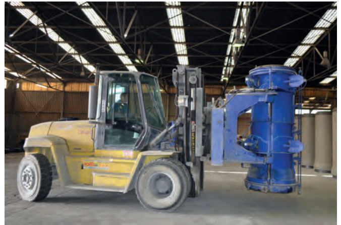
Fork-lift truck with a 3-part mould jacket
