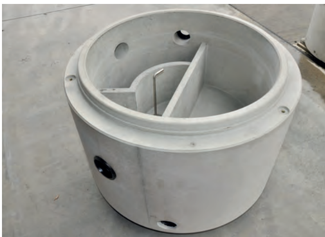
DN1200 water chamber manufactured from flowing concrete with individually moulded channel and gaskets encased in concrete.
