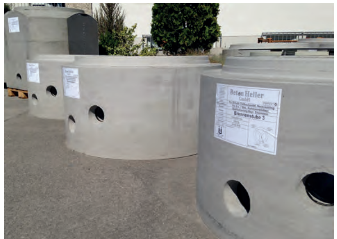
Concrete water chambers with seals and overflow shafts integrated in the plant produced by Beton Heller, shortly before being shipped to the construction site.
