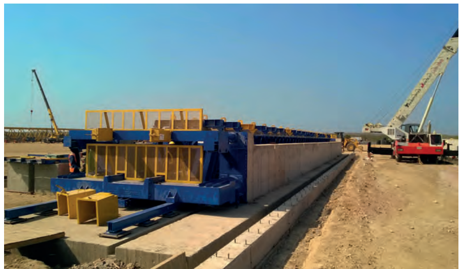
The 40 m mould was installed in the vicinity of the construction site. It can be used independently of location, since it has a self-stressing system.
