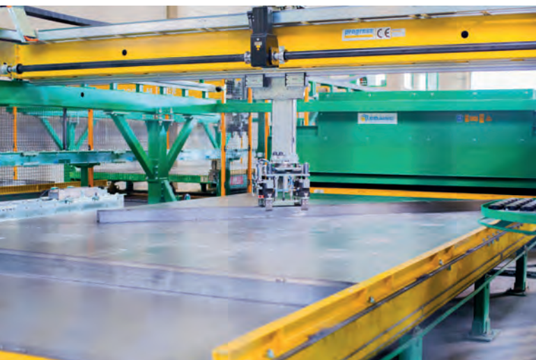
Six minutes: the time required for the shuttering process has been significantly reduced by sophisticated robotics and software.
