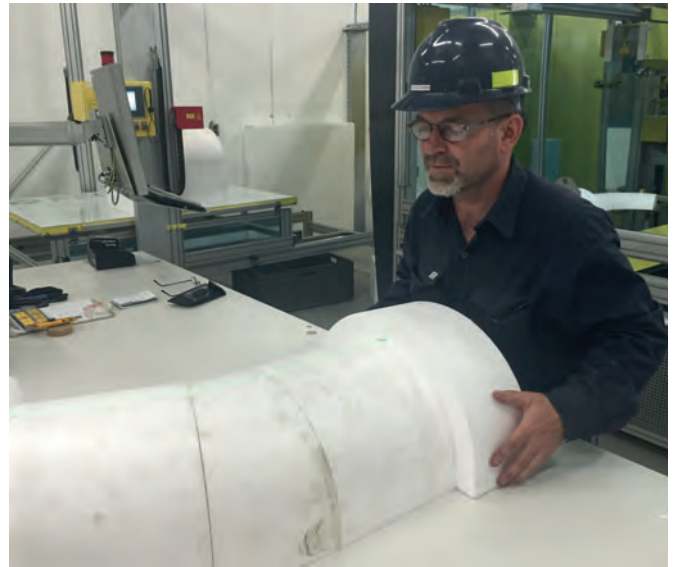
Positioning lasers are used to help the worker to assemble the negative channel, while at the same time providing quality control.
