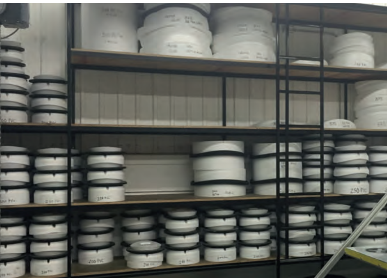
Pipe connection form parts, cut to size from polystyrene rigid foam using a profile saw, with fitted gaskets.
