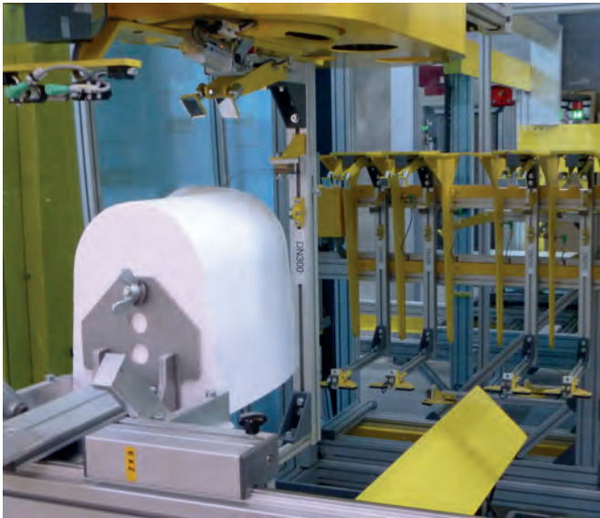
One of the characteristics of the Perfect system is the computer-controlled hot wire cutting technology, which ensures the precise cutting of the negative channel components and the pipe connection form parts.
