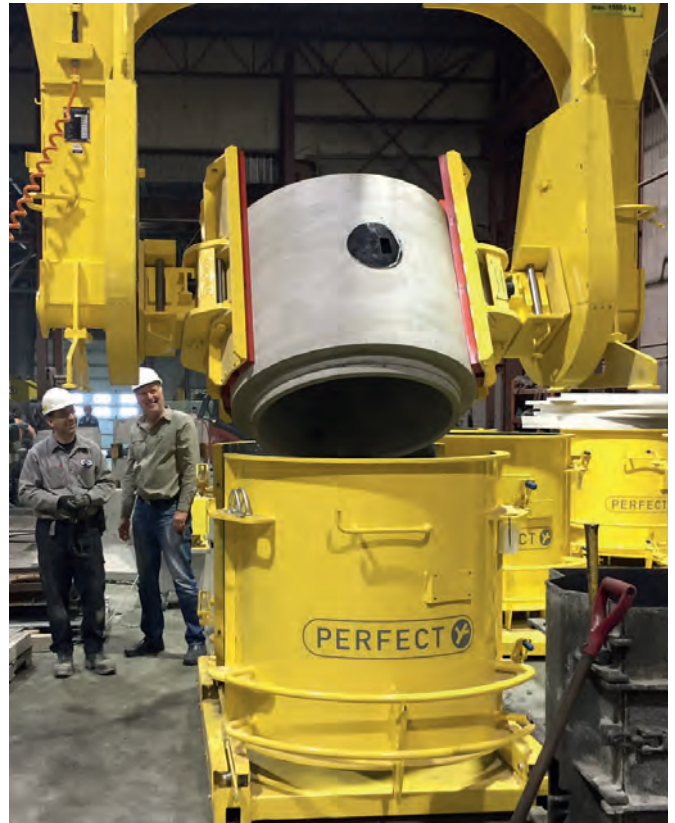
The finished monolithic manhole bases are lifted with the help of a product gripper and rotated 180°.
