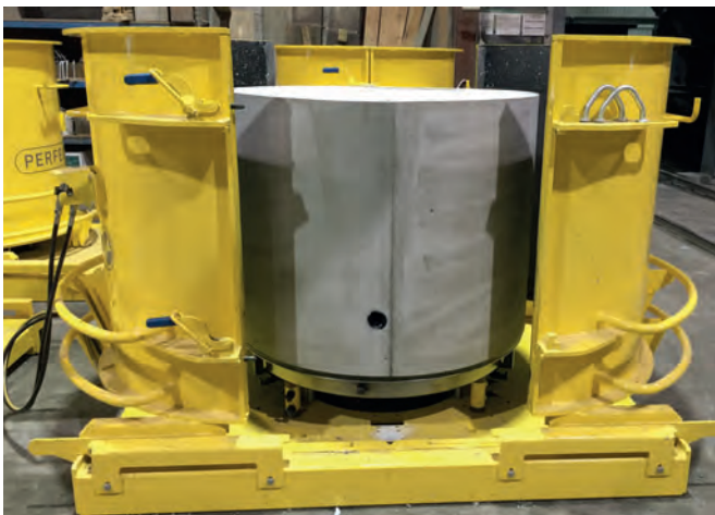
At Fortier 2000 Ltée, the manhole bases, which are manufactured from self-compacting flowing concrete, are usually demoulded the following day.
