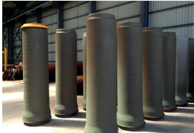
The freshly demoulded pipes usually remain in the curing area of Trans-Canal Centre for one working day.
