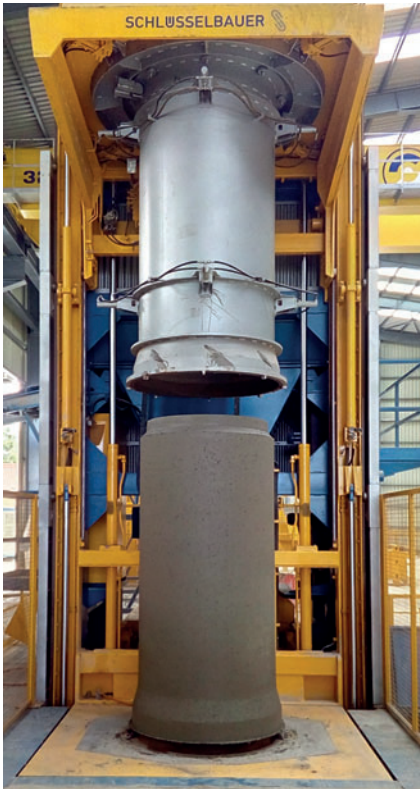
Production of a DN800 bell sleeve concrete pipe using the Precise system supplied by Schlüsselbauer Technology.
