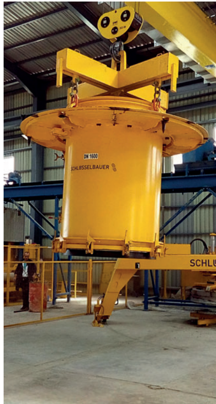
Feed pipe of a prepared steel mould on the Exact XL production system.
