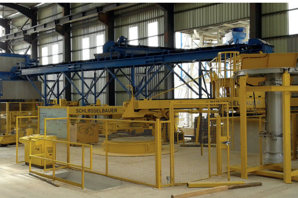
Exact XL automatic pipe production system in the concrete factory of Trans-Canal Centre in Algiers.
