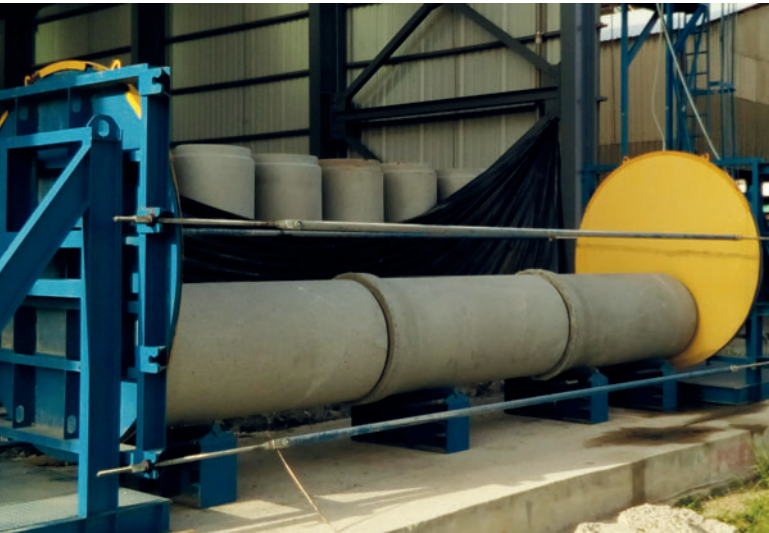
The concrete pipes produced on the Exact XL and Precise machines are tested for watertightness and load capability.
