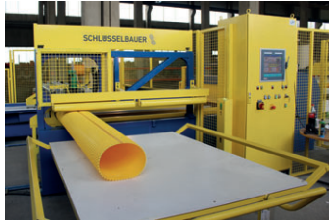
With the help of a robot, a welding seam is created using PE wire to establish a solid connection between the two ends of the foil. After welding the foil has transformed into a Liner-cylinder.
