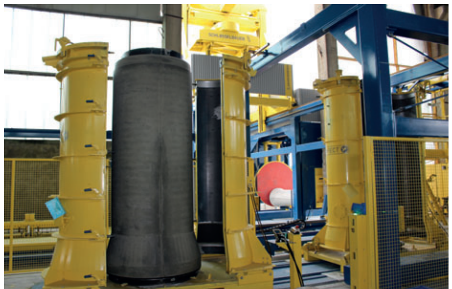
The pipes are carefully released and lifted up from the mould core by a robot equipped with a universal gripper for all pipe diameters.
