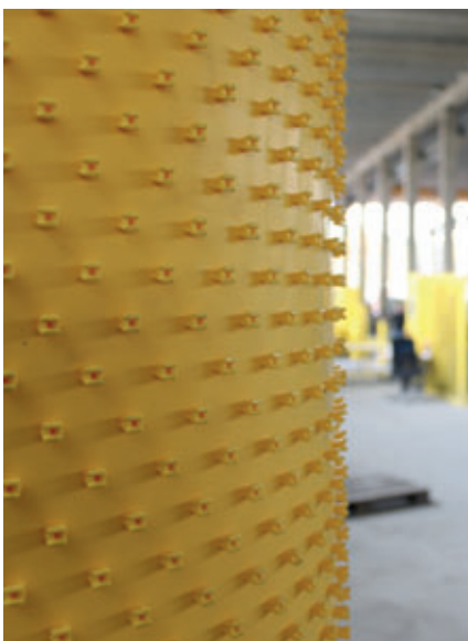
The tight connection of the Liner with the surrounding concrete in the subsequent pipe is guaranteed by multiple anchoring points at the back of the Liner-cylinder.
