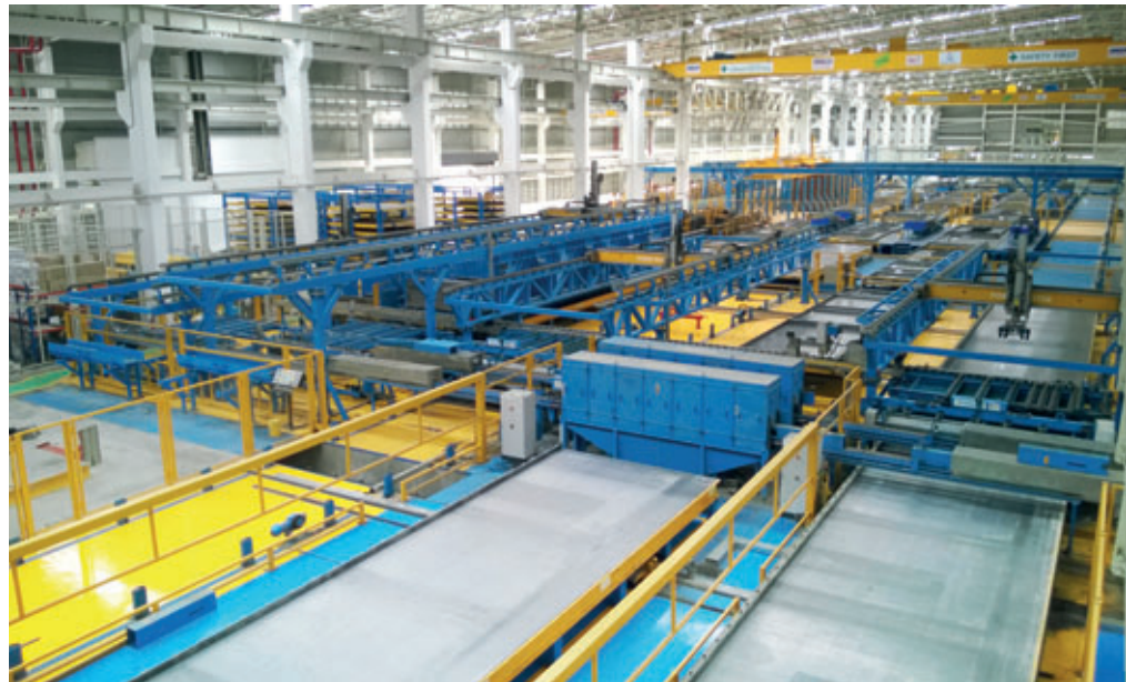
View inside the new high-performance plant at Pruksa: the demoulding and shuttering of the pallets as well as the cleaning and oiling of the pallets and required shuttering elements are completely automated.
