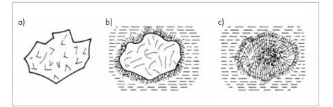
Chemical Cement Hydration Process: seen here, the importance of moisture on cement hydration. a) Cement grain prior to the addition of water
