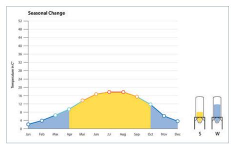
Due to seasonal changes in the ambient temperature and its affect on the speed of concrete hardening, cement content is raised/lowered in order to achieve the necessary early strength in order to cube.
