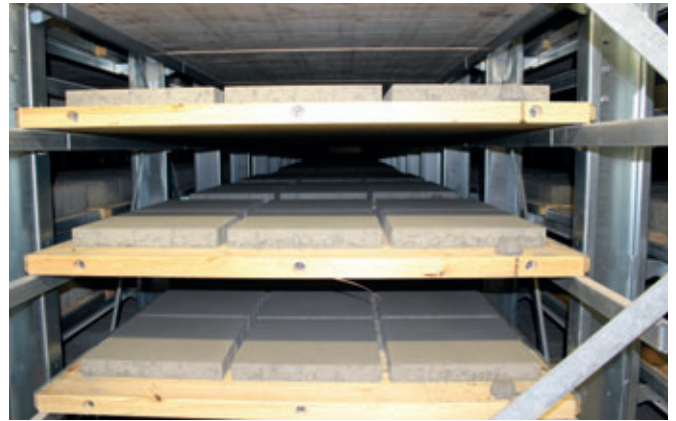
The curing rack – a giant-sized climatic chamber
