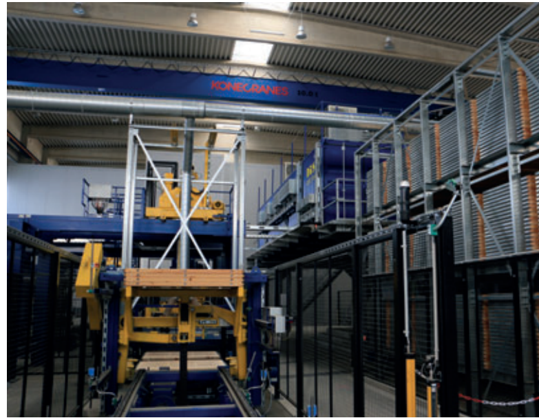
Masa chain conveyor for stacking production pallets
