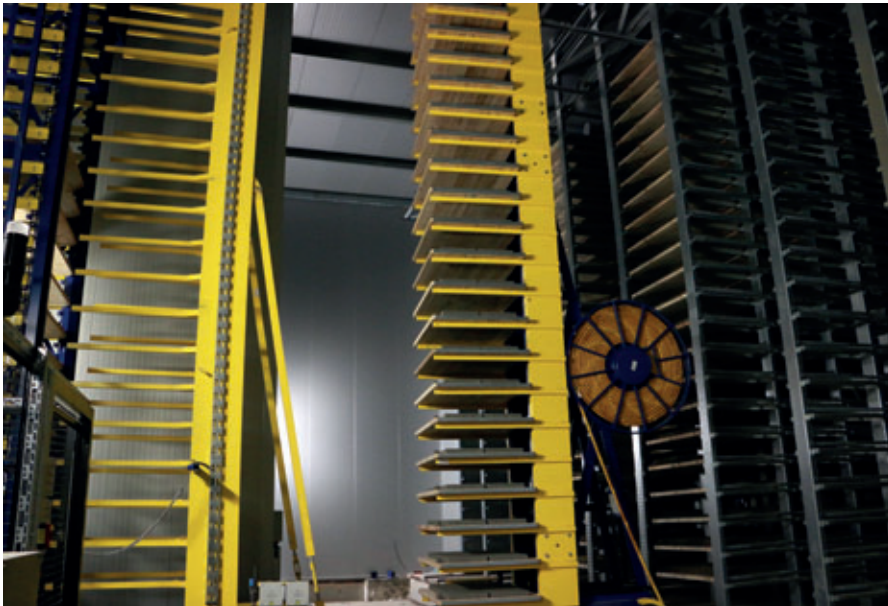
Transfer table and finger car system with intermediate storage
