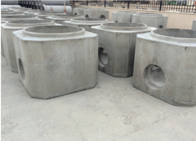
Finished manhole base components with formed inlets and outlets
