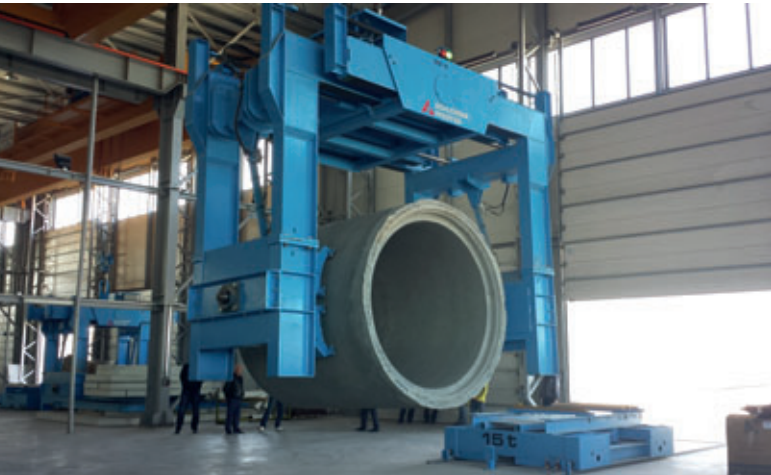
Grab for turning pipes with products up to 15 tonnes in weight
