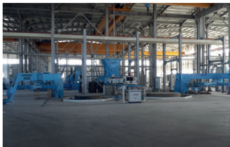
Prinzing-Pfeiffer Variant 3600/2500 for concrete pipes up to a 3,600 mm and lengths up to 3.0 m
