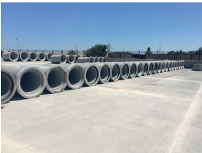
Finished reinforced concrete pipes before delivery to customers
