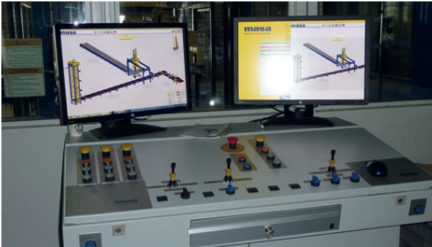
Always everything in focus: Due to the modular plant control software Masa FAST
