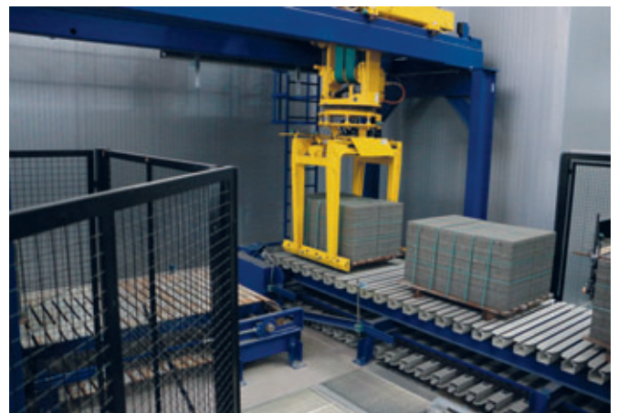
Another Masa transfer unit takes the strapped packages of blocks and places them on a package conveyor set up at an 90° angle
