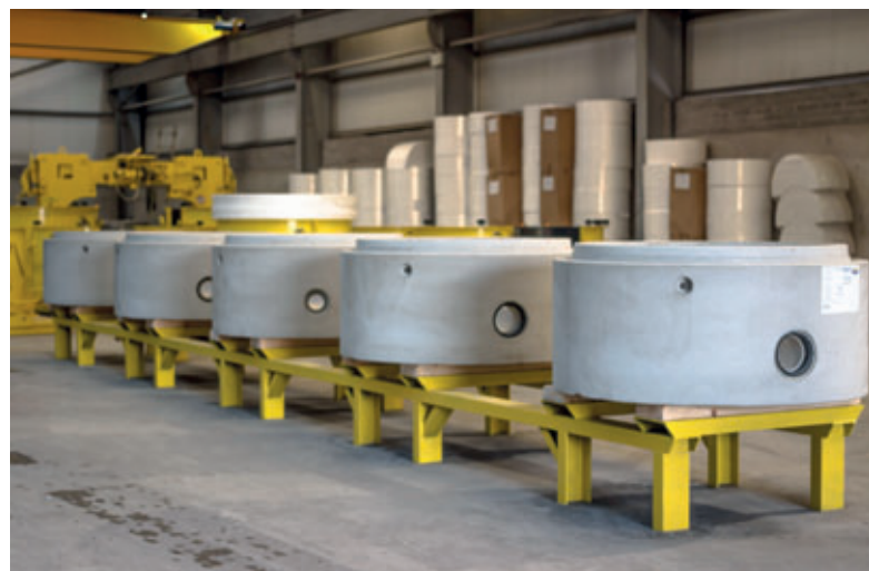
Monolithic concrete manhole bases with individually tailored channels from the current production.
