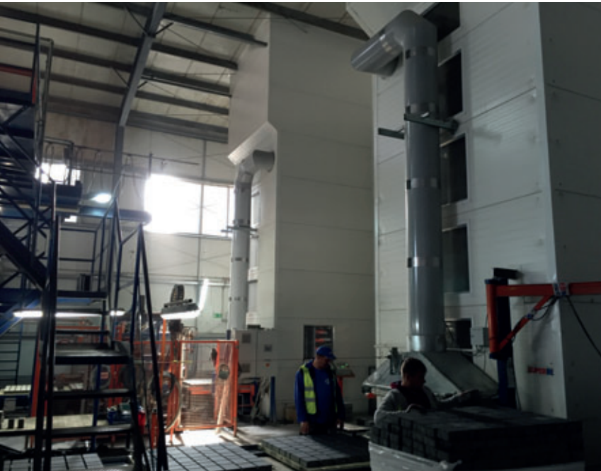
Quadrix 300-150 Heating & Air Circulation Unit with Nautilus™ air distribution duct prior to and after
