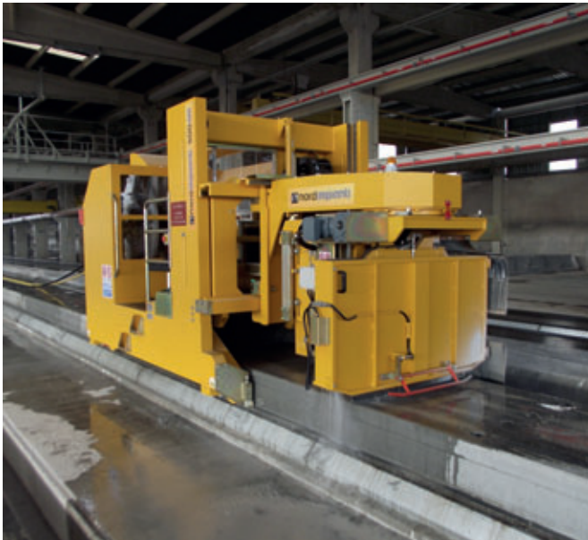
500 AM Multi Angle Saw during cutting of the manufactured slab.
