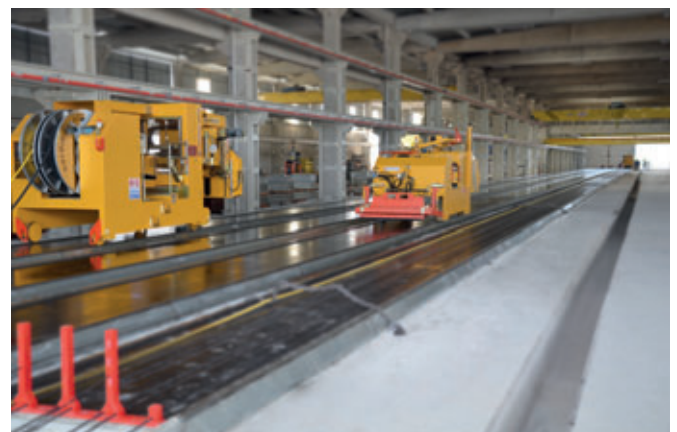
Interior view of the new production area for hollow core slabs in the Kambeton prefabrication factory.
