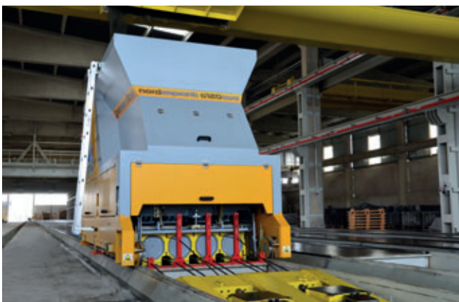
The Nordimpianti EVO e120 Extruder, capable of producing hollow core slabs with heights of 150, 200, 265, 320, 400 and 500 mm.
