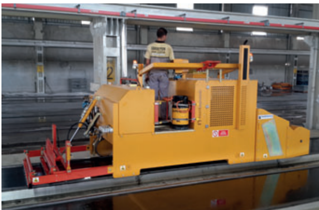
Multi-function bed cleaner during production bed preparation.
