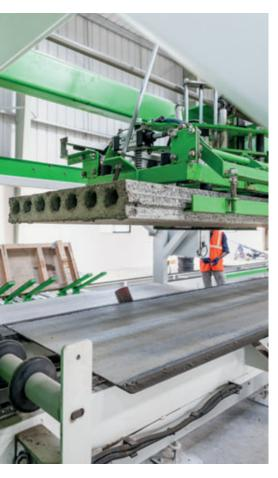
Elematic Acotec production line is meant for manufacturing of light, non-load bearing, room-high precast partition wall panels. The line covers the entire production process from concrete batching all the way to storage yard management and beyond.
