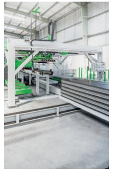
All Acotec wall production lines feature a new advanced production control system and a simple, modern user interface that shows detailed data on every function in the whole process. Various reports – on production rate, running hours and more – are also generated automatically.
