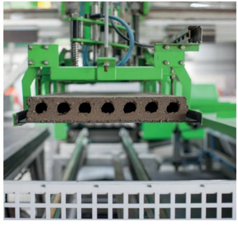
Industrialized production process of the Acotec line translates into high quality that shows in exact panel dimensions and flat panel surface.
