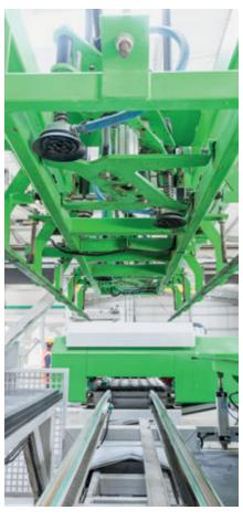
Modular structure of the Acotec lines and their integrated electricity with Ethercat bus system guarantee short installation and start up time of all lines. The line can also be installed in existing production facilities
