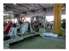
The two wheels of the VTA are electronically synchronised; the Progress inverter welding provides quality and efficiency.
