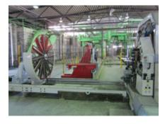
Following production the finished reinforcement cages are automatically removed.
