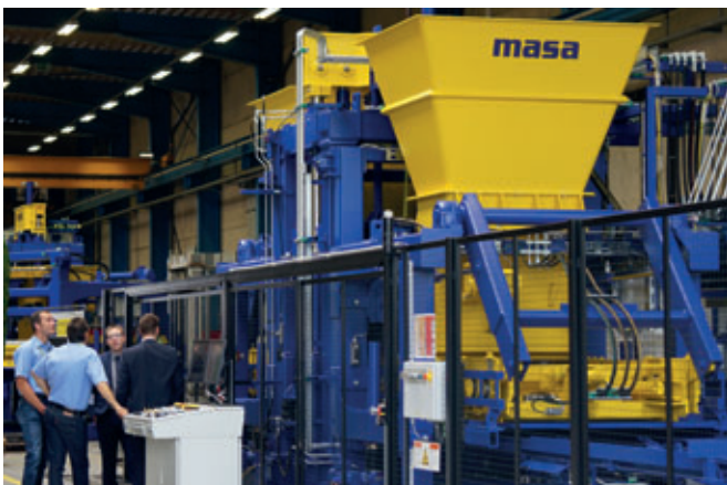
The machine demonstrations were a special attraction – In addition to the Masa concrete block making machine XL 9.2 ...
