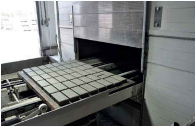
Fresh concrete products pass through a small adjustable opening in the curing chamber wall within 30 seconds of being produced – eliminating evaporation of moisture from the concrete. "Our machine operators say: the edges are now perfect!"
