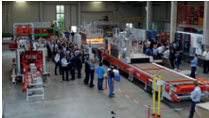
Presentation of the universal print-coating line for concrete pavers and panels during the in-house trade fair at SR-Schindler
